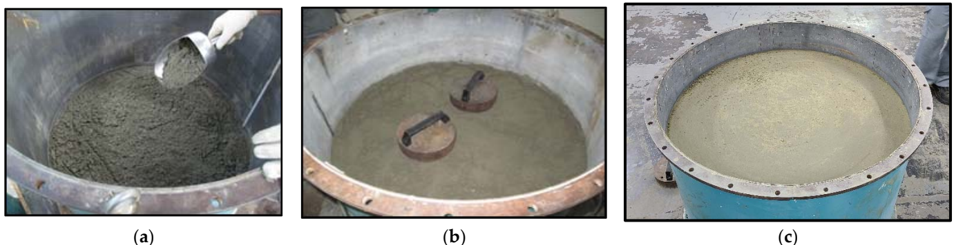
Figure 4. Soil foundation setting: (a) soil sprinkle; (b) soil compaction; (c) soil foundation set-up.
