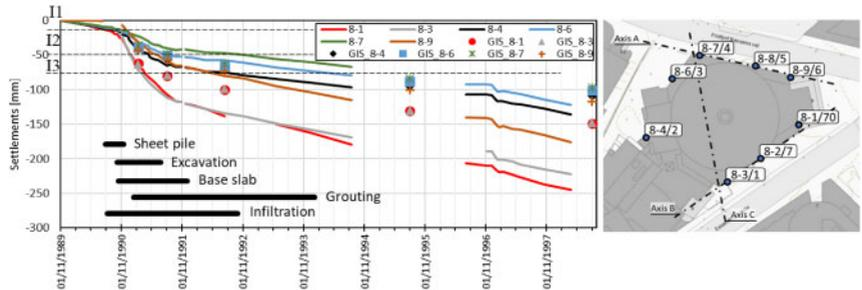
Figure 10. Comparison between predicted and measured settlements. Continuous line: measured settlements of the Colosseum cinema between 1990 and 1999. Point: settlements of the corners point of Colosseum cinema at 4 different time steps: 0.1, 1, 2, 5 years, calculated with the GIBV tool. Position of settlement bolts shown on the right.
