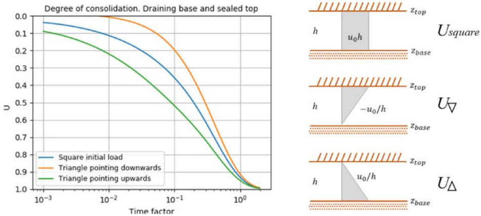
Figure 5. Triangular isochrone and corresponding U-T curve (from Terzaghi & Frölich 1936)
