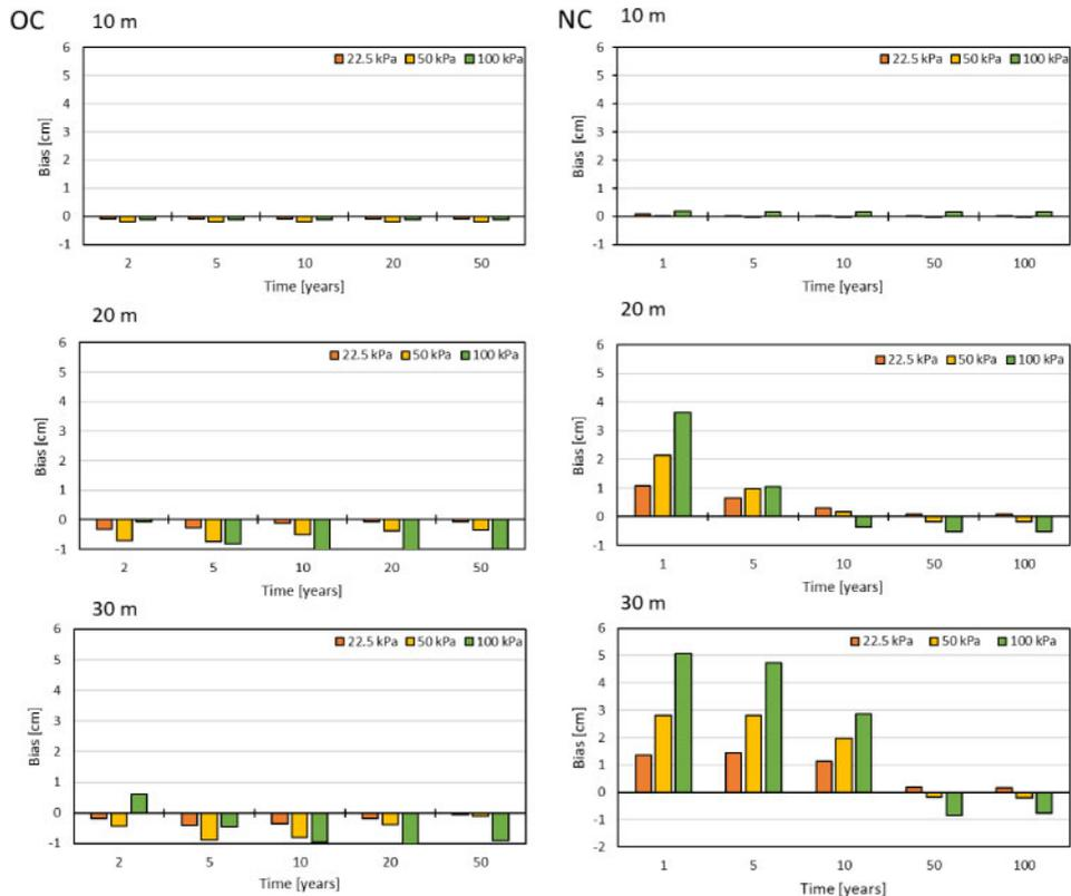
Figure 7. Differences (bias) between settlements computed by the GIBV methodology and Geosuite calculations for the scenarios described in Figure 6.
