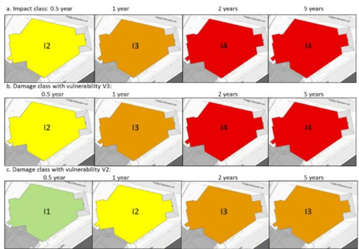
Figure 11. (a) Impact class in time considering the maximum vertical settlement ( $\delta v, max$ ) experienced by the corner points of Colosseum cinema. Damage class in time with a vulnerability class V3 (b) and damage class in time with a vulnerability class V2 (c) for the Colosseum cinema due to the excavation.
