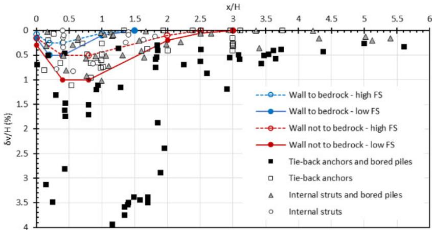
Figure 2. Expected normalized settlement,  $\delta v/H$ , versus normalized distance from wall,  $x/H$  in clay soils using different support methods.
