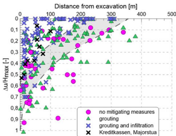
Figure 3. Database of pore water pressure reduction due to excavation works in Norway:  $\Delta u$  = pore water pressure reduction in m measured at the base of clay stratum,  $H_{max}$  = depth of excavation base beneath initial ground water surface (adopted from Langford et al. 2016b).
