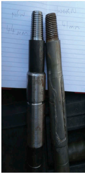
Figure 7. New rod with friction reducer 44mm left and to the right the wear has reduced diameter to 41 mm and in parts of the FR it is ripped off completely.
