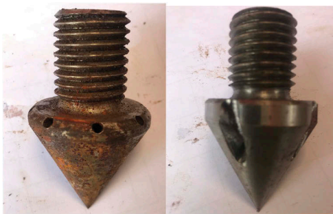
Figure 3. Various cone tips with water flushing for DCPT cones.
