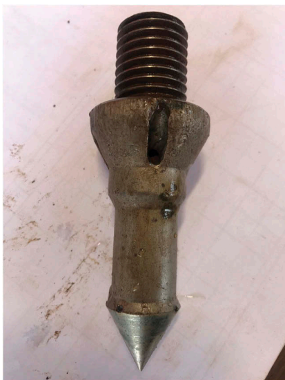
Figure 5. Instrumented cone tip used with the iDCPT.
