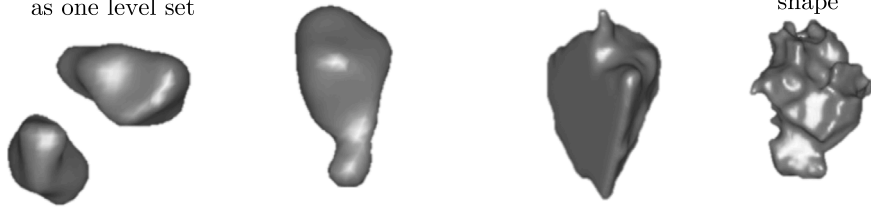
Fig. 5. Types of defects in the image segmentation process described by Fig. 4 to go from raw 3DXRCT images of a real sample of Jaramijó's soil to individual level set-based digital grain avatars: (a) Individual parts are given the same label during the semantic segmentation process, and finally coming up as one level set function, (b) typical undersegmentation case caused by different grains in contact being recognized as a single one, (c) typical oversegmentation case caused by a single grain split into several parts, and (d) unrealistic shapes caused by the detection of voids, noise, or grain clustering. From 2935 digital grain avatars, 45% of them display some kind of defect, and 55% corresponds to the properly processed digital avatars.
