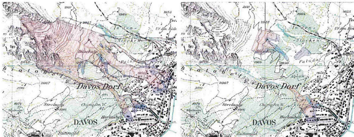
Figure 6.7 Left side: Worst-case scenario without avalanche defence structures, similar to the 1919-avalanche event. Right side: Avalanche hazard map 1999: Worst-case scenario with avalanche defence structures.
