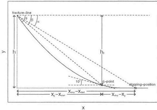
Fig. 1. Definition of geometrical parameters used to analyse extreme runout.
