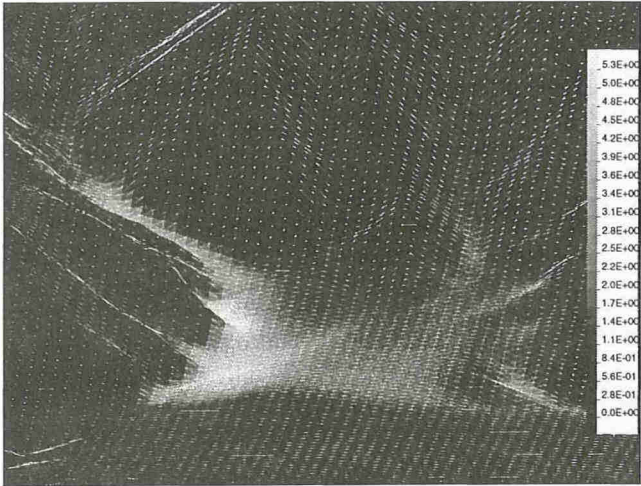
Figure 4: Avalanche flow height distribution [m] in the Arelen track at the entrance into the runout (60s after the release). Perspective view from east to west (see Figure 5). Topographic Data: © Swiss Federal Office of Topography.
