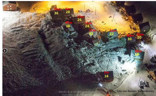
Figure 5: House number (yellow) and preliminary measurements of distance moved (red). Photo: Svalbardposten.
