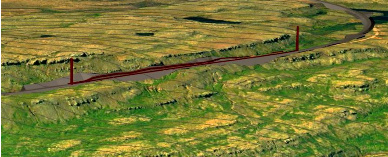
Fig. 4. This aerial photo is draped on a digital terrain model (DTM). The observation site is between the red vertical lines. Above the road is a rock wall, steep scree and cliffs; below is the road fill. Wind direction lines of 22^\circ (NNE) are draped on the terrain model. The distance between the lines is 50 m.
