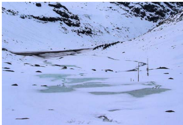
Fig. 3. A picture from a time-series of water level fluctuation in snowpack on uneven sloping ground. Snow-height variation 1.5-3 m. NGI field station May 16 20:24, 2010. (Photo K. Kristensen, NGI)
