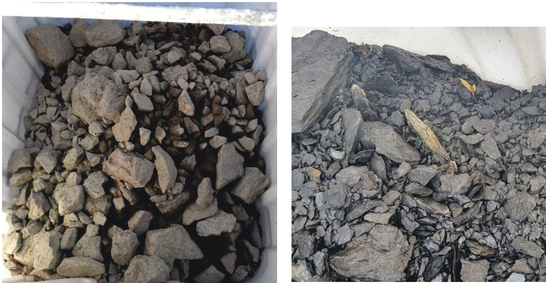
Figure 11 Content of container with 100 % rhomb porphyry to the left and alum shale to the right
