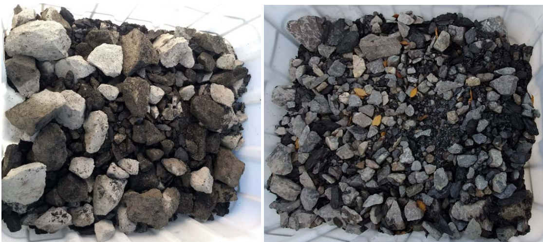
Figure 7 Content of container B10_1 (10 % alum shale, left) 13.10.2020, and B20_2 (20 % alum shale, right).
