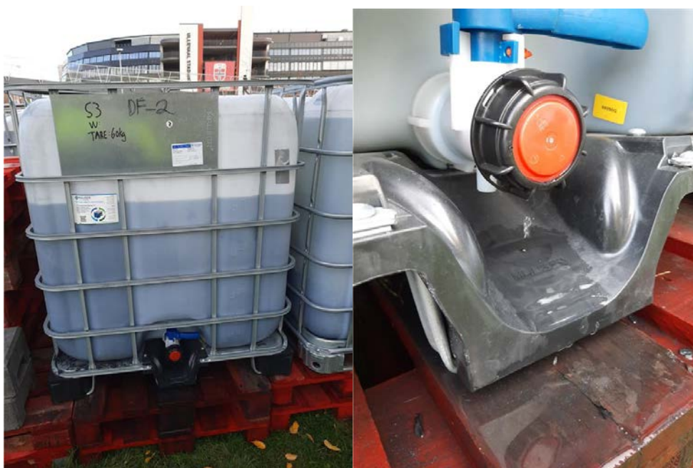
Figure 10 Missing water in DF_2 container (left), and water running from the tap of the same container (right). Photos taken 05.11.2020.
