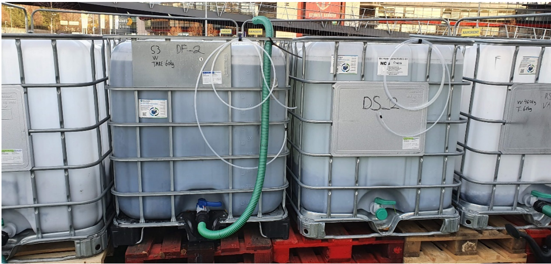
Figure 5 Alum shale containers filled with freshwater (DF_2, left) and saltwater (DS_2, right) for investigation of underwater disposal. DF_2 was leaking from the tap and a tube was put on to stop the leak.
