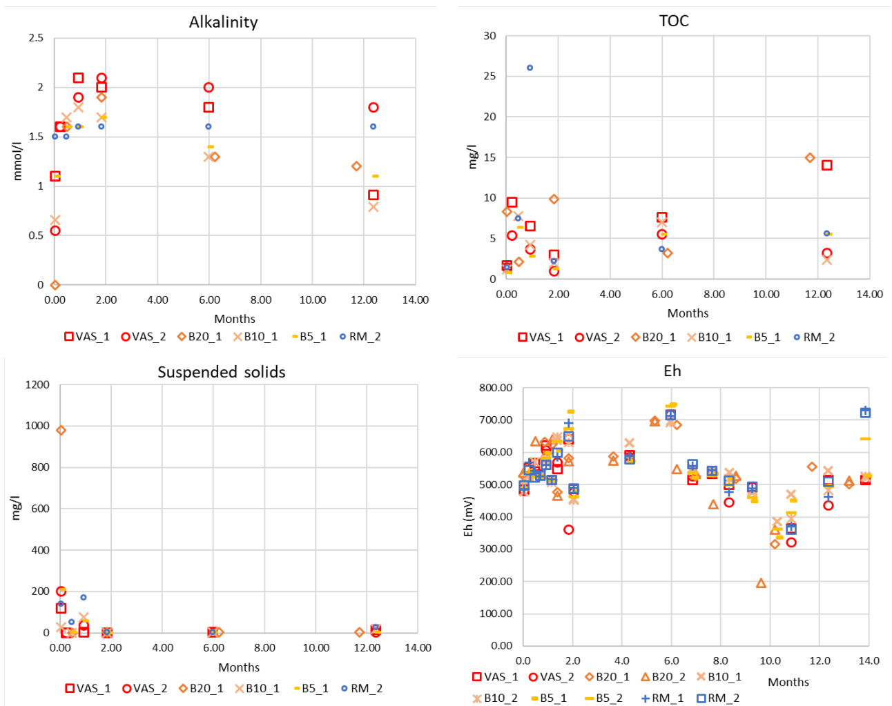
Figure 27 Alkalinity, TOC, E_h and suspended solids (SS) for the first ~12 months of the containers experiments with alum shale from Kleggerud mixed with rhomb porphyry. VAS = pure alum shale, RM = rhomb porphyry, B20 has 20 % alum shale etc. Except for VAS, only one replicate container was measured, as can be seen from the legend.
