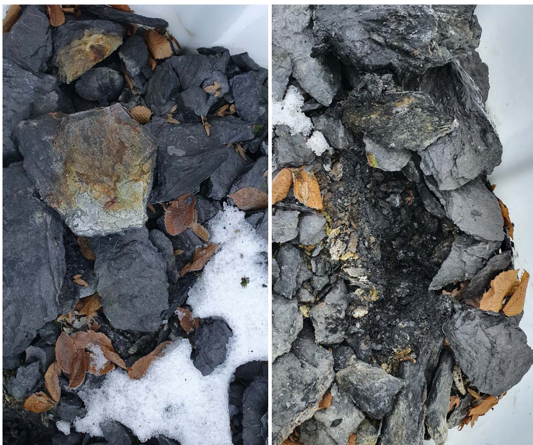
Figure 61 Photos from A1 taken 17.12.2021. When lifting the larger rock pieces, we see precipitation products and weathered rock material (sand sized) underneath.
