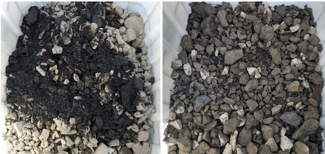
Figure 6 Content of container B5_1 (5 % alum shale and 95 % rhomb porphyry before (left) and after (right) mixing of the rock masses. 13.10.2022.
