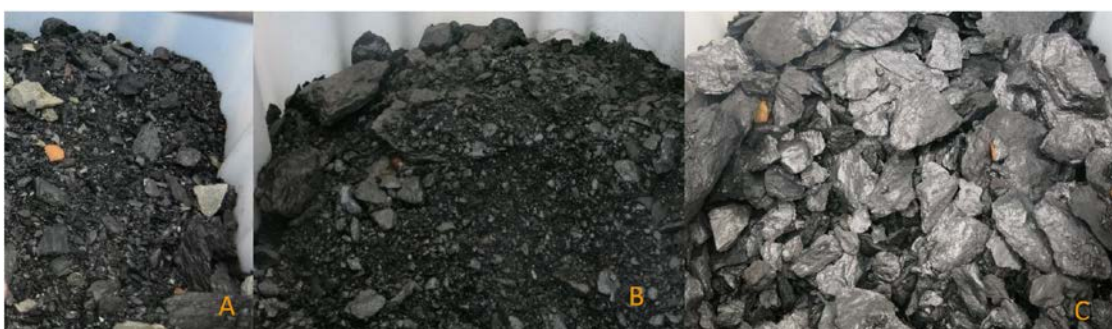
Figure 15 Rock masses used in containers set up in 2014, taken in the containers 2 weeks into the experiment. A) Galgeberg shale collected from the tunnel (G2). B) Alum shale collected from road cut (A3). C) Larger pieces of alum shale collected from road cut (A1). Photo copied from figure 3 in SVV (2017).
