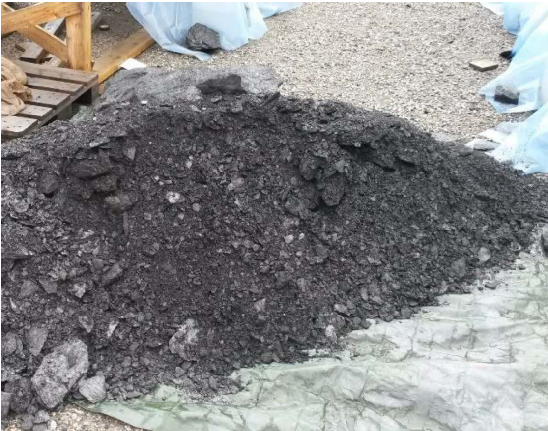
Figure 16 Alum shale from tunnel, used for the experiments started in 2015 (AT1 and AT2). Photo copied from figure 4 in SVV (2017).
