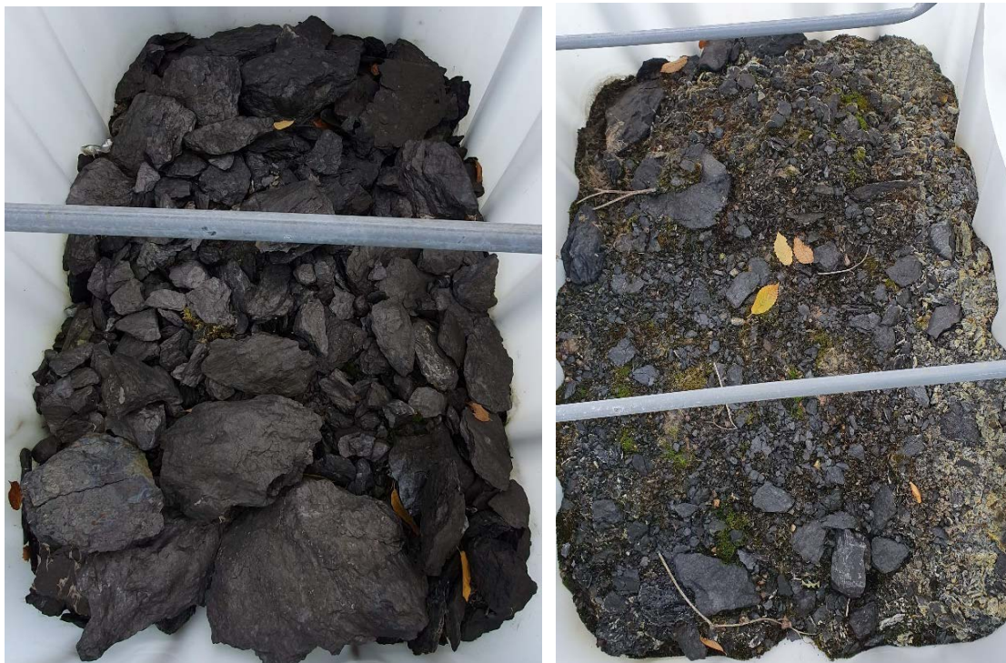
Figure 52 Content of container A1 (left) and A3 (right), taken 19.11.2020, after the containers were transported to NGI, 6 years after experiment start up. The green is moss while the white/yellow is precipitates, likely iron sulphates.
