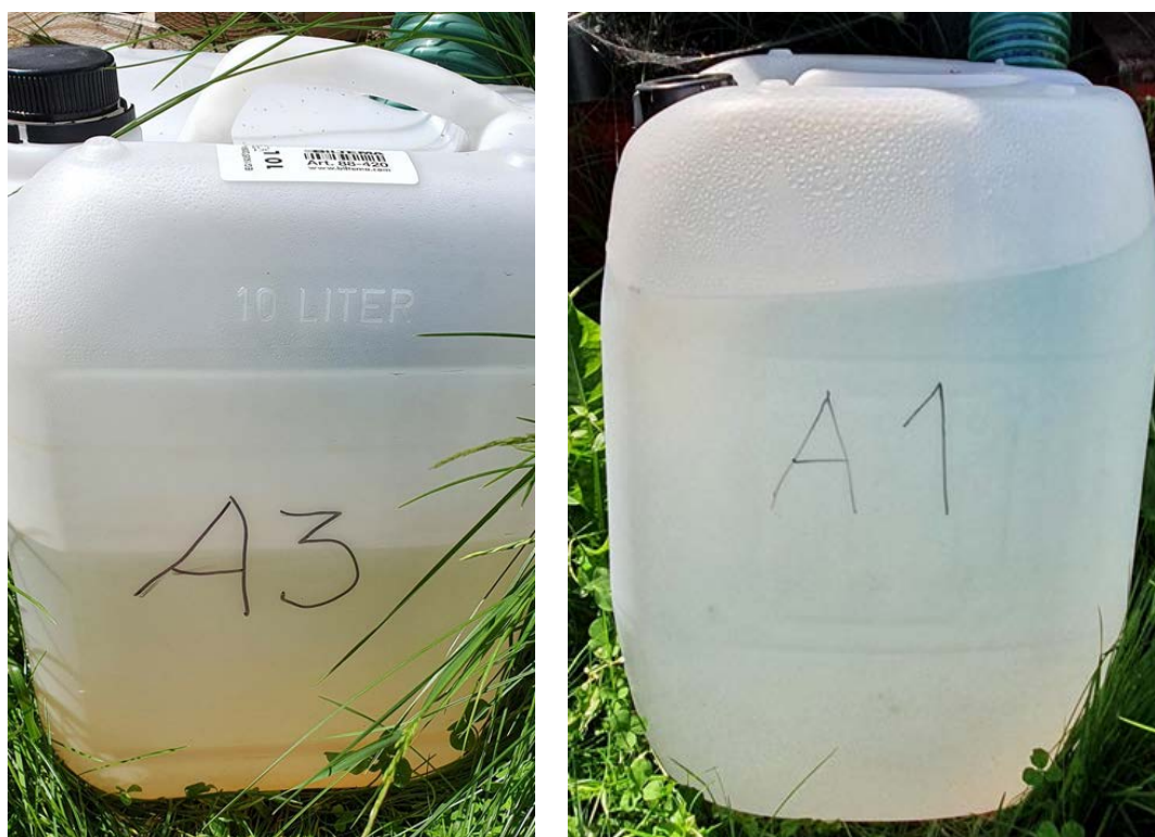
Figure 59 Iron precipitates in canister collecting water from SVV container A3, but not from the A1 container that has rock from the same road cut but larger pieces. (Photos taken 23.06.2021).
