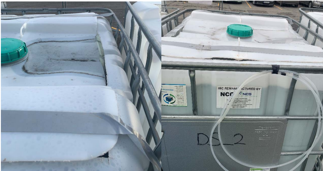
Figure 12 Photos taken 01.03.2021 shows that rainwater could leak into containers.
