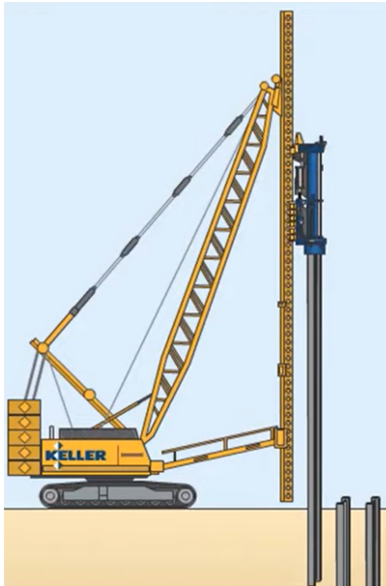
Figure 8: Establishment of Steel Core Piles [20]
