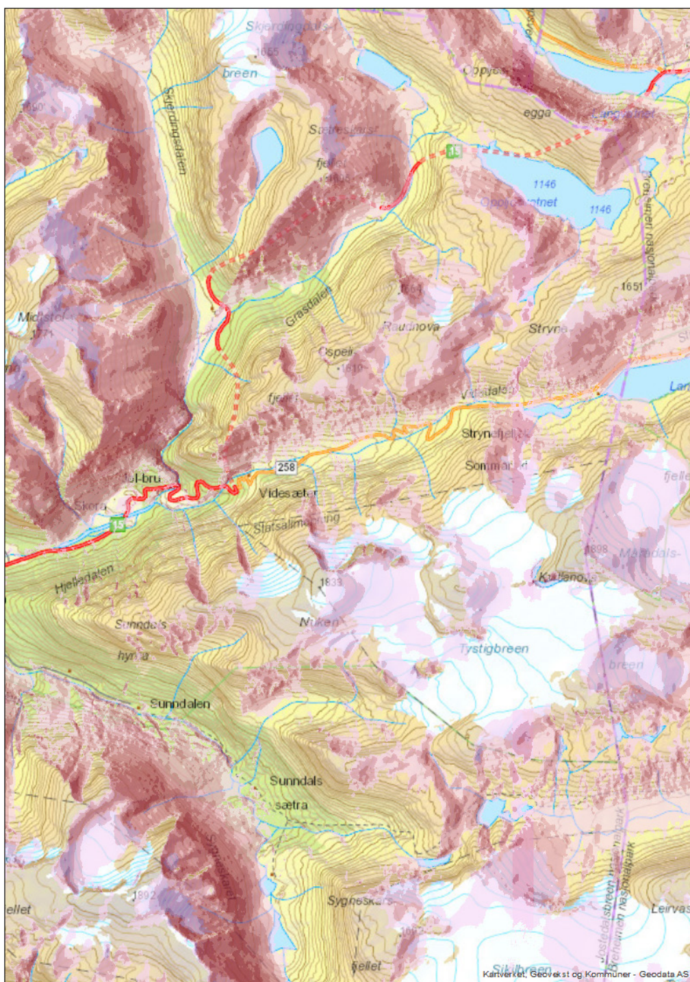
Figure 31 Winstral sheltering index for wind from west (270°) applied on the national 10 m DEM from the Norwegian Mapping Agency for Strynefjellet. Darker red colors indicate higher degree of sheltering and therefore areas more prone to snow accumulation
