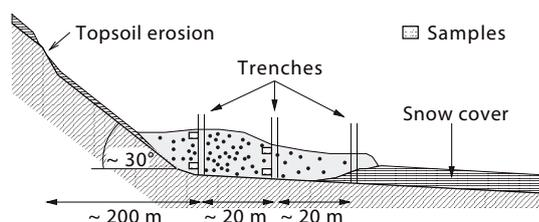
**Fig. 4.** Schematic longitudinal section of the deposit of the 21 February 2006 avalanche at Sertig Dörfli, indicating the location of soil erosion, the placement of trenches and the soil concentration in the deposits.
