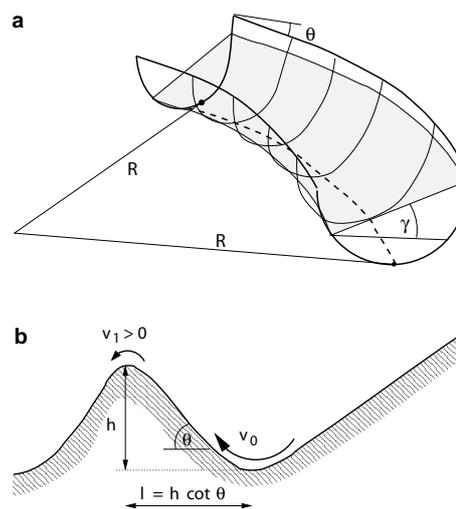
**Fig. 3.** (a) Superelevation in a bent gully. The curvature radius of the centre line is  $R$  and its inclination  $\theta$ . The idealized flow surface is inclined by the angle  $\gamma$  relative to the horizontal. (b) Schematic drawing of moraine overflowed by the fluidized head of the 22 January 2006 Kreuzweg avalanche.
