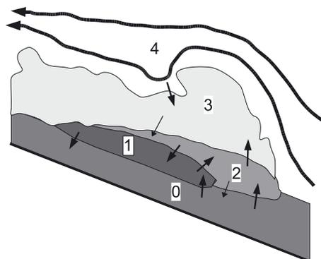
**Fig. 1.** Schematic representation of the structure of fully developed dry-snow avalanches with (1) dense, (2) fluidized and (3) suspension flow regimes occurring simultaneously. Arrows indicate mass exchange between the layers, including the snow cover (0) and the ambient air (4).
