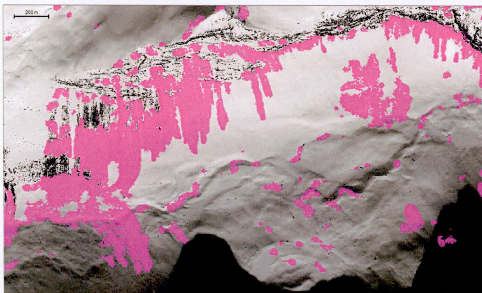
Figur 4. Identification of snow avalanches in a WorldView-1 image using an algorithm developed for Leica ADS-40 imagery.
