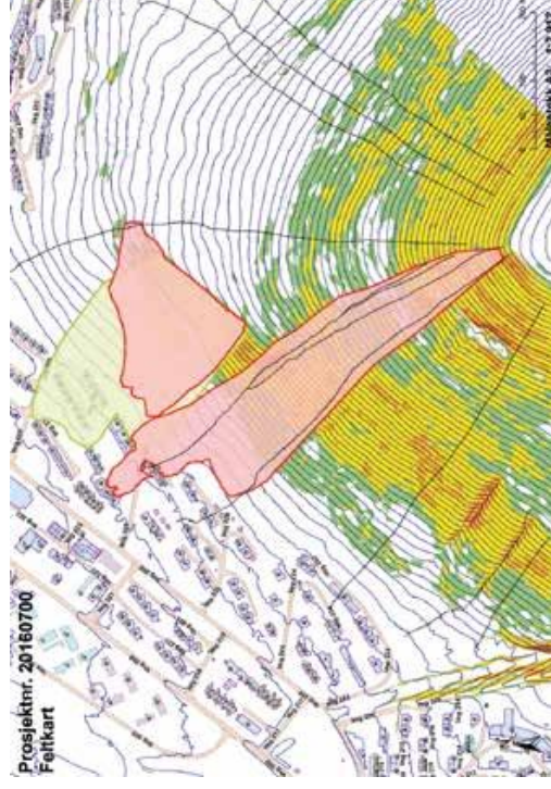
Fig. 4: Overview over the avalanches from Feb. 2017 (in red) and Dec. 2015 (light green). Black lines indicate fall-line (steepest line). Slope map: green indicates 27°-30°, yellow to red is steeper. Contour line equidistance is 5 m. Adapted from (NVE, 2017).
