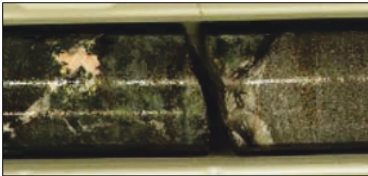
Figure 7. Low friction joint at 91 meters.
