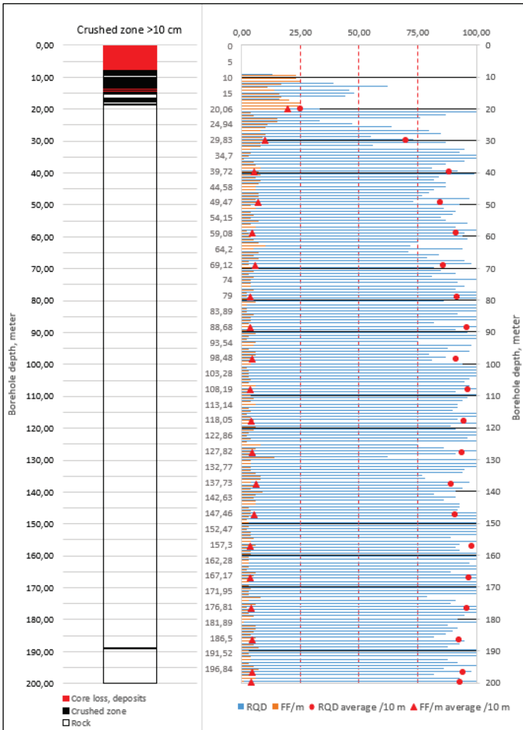
Figure 3. Simplified overview of RQD, average RQD every 10 meters, FFm, average FFm every 10 meters, crushed zone >10 cm and core loss distribution in KH-02-18.
