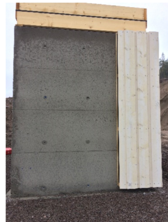
Figure 1. First blast test a) Test area (left) and test buildings (right). The casted concrete building is under construction. b) Leca building with plaster on outside. c) Inner wall of Leca building covered with tiles (the outside of this wall was facing the blasting area). d) Wooden panel mounted on one corner of the concrete building facing the blasting area.
