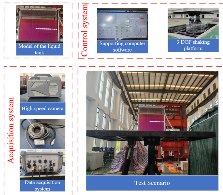
Figure 2. Operational diagram of the sloshing test system.
