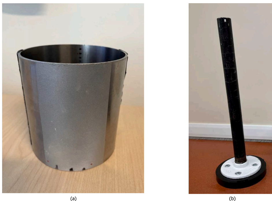
Fig. 2. a) Photo of the steel cylinder used for compaction. b) Photo of the compaction apparatus used to compact snow within the steel cylinder.
